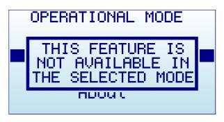
If your analyzer includes two modules (e.g. ISM Combo) only one of the modules may be the one with the available functionality. Make sure to select the right module before trying to use the functionality (e.g. the ISM Combo has the 2.4G module enabled on the SMA module at the right) otherwise above message will popup.
