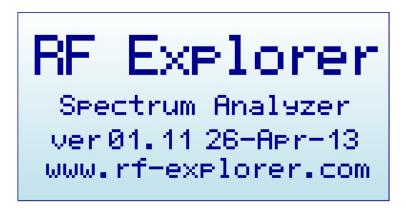
**Note**: if you enable this screen for more than 30 seconds while connected to USB port and power switch in the unit set to ON, RF Explorer will automatically go to low power mode and will switch the LCD off, but will keep charging the battery. This is suggested when you intent to charge the internal battery but not make use of the unit for measurement.
