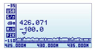
**Note**: While RF Explorer Spectrum Analyzer screen is enabled, the [Left] and [Right] buttons can be used to increase or decrease the Start/Stop frequency, virtually moving the visible spectrum to the left or the right 25% on every key press. This is helpful in order to offset the visual range without need to specify a new numeric range.
